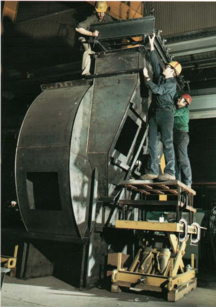
Fans designed for field erection are first fully assembled at the factory to guarantee accurate fit-up at the jobsite.
